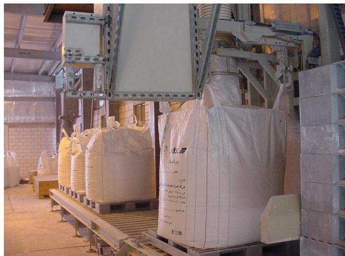
Bags being filled on the IBC-PF4 and being transported along the conveyor
