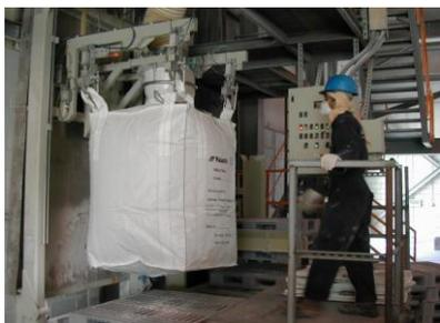
Protective masks, goggles and suits are worn to ensure the silica flour is not inhaled.
