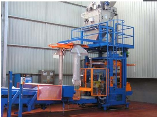
*Form-Fill-Seal bagging. High Speed packing of 5-25kg bags*
