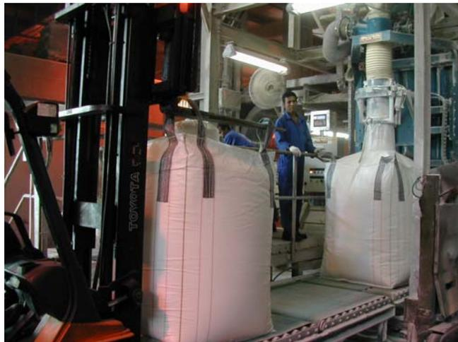
The two 50kg bagging lines pack two different grades of sugar into 50kg bags.
