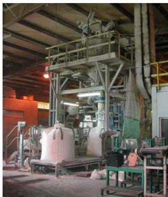
The filling spout on the IBC-PF2 machine was supplied with pneumatically operated flaps which close at the end of the filling cycle to prevent any residual product from dropping onto the top of the container as it is removed from the filling position – resulting in a clean, secure bag which is essential in a warm climate.
