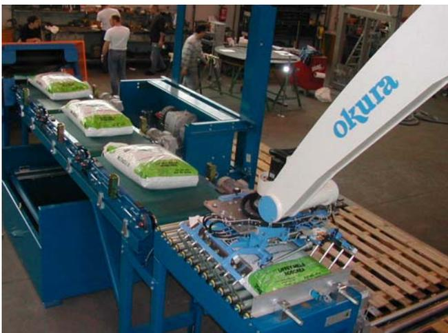
*Pictures show various views of the Webster Griffin system - Okura robot palletiser (this page) and (overleaf) the automatic pallet wrapper during factory test*
