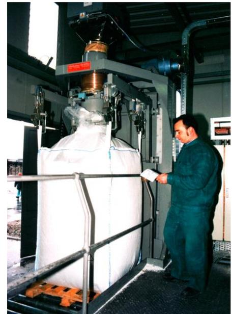
An RS232 output links the weighing system to a barcode and label printer, a printed label is placed in a pocket on each bag and displays a unique bag identification number, as well as the final customers name, product grade, batch number, date, time and the actual net weight of product in the bag
