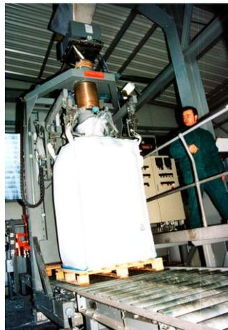
Owing to the high value of PET resin at up to US\$2,000 per tonne, Italtip Preforme needed to reduce product give away and stipulated an accuracy of +/- 500g - 1000g/bag dependable accuracy is ensured by Webster's 'self optimising' digital weighing controller, via a 'Querty' keypad the weighing system can be loaded with 100 different sets of instructions for different bag weights and product bulk densities, these pre-set instructions are re-called by entering an alpha numeric code.
