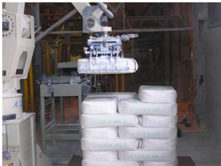
Following evaluation of various robots, an Okura A400 series III robot with OXPA "Easy Teach" programming system was selected.
